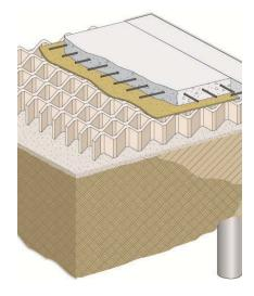
GeoVoid design for each application is determined based upon the thickness (t) and depth (d) of the GeoVoid compressible fill material.
